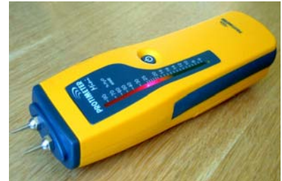
Fig 1: GE Protimeter resistance type pocket size moisture meter
